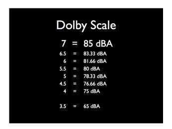
The picture above shows the scale of the Dolby box volume control. The reference noise is 85 dBC at "7", 80 dBC at "5.5" and 75 dBC at "4". Below 4 the scale becomes 10 dB per 0.5 step. At 3.5 the ref noise is at 65 dBC. From the Dolby CP650 manual I quote:
