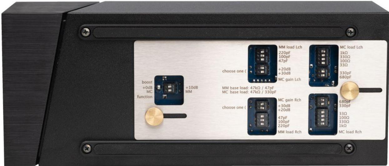
MM cartridges can use capacitances of 47 pF, 100 pF, or 220 pF. Some manufacturers offer even higher values, but Grimm feels that this is unnecessary. Higher values, such as 1000 pF, can create unwanted peaks in the frequency curve.
