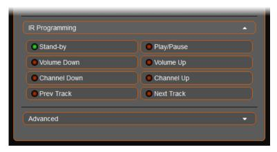
The infrared remote functionality requires an IR extension cord connected to the 3.5mm jack on the back. Please see the hardware manual for the connector location and pinout information.
