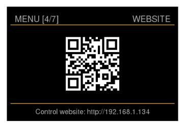
This menu shows the information you need to connect to the Grimm User Interface (GRUI). The GRUI is the web control interface of the MU1. You can scan the QR code with your tablet or mobile device. As an alternative you can manually enter the link shown at the bottom of the screen in your browser. More information about the GRUI can be found in chapter GRUI MU1 Web Control. This menu page will always be shown at maximum screen brightness for optimal scannability.
