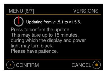
Please note: depending on the type of update the install can take up to about 15 minutes. During this time you will not see information on the display, the power LED is fading quickly<sup>1</sup> and the power button on the back is disabled. **Please remain patient and do not unplug the device while updating** since this causes the update to fail and the procedure has to start again when the device is powered up.
