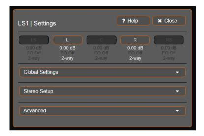
The first row shows a summary of the setup data per LS1. In the top row you see buttons with the names of the detected speakers. You can press these buttons to mute the indicated channel for a few seconds. This LS1 will blink its power LED, so you can easily identify the speaker and see if the wiring and LR switches in your system are correctly set.
