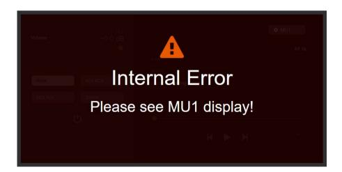
The MU1 does a self-test to guarantee the FPGA conversion quality. Whenever something is wrong it will instruct you to do a full power cycle by pressing the main dial. The unit will then shut down. Please wait until the MU1 is completely shot down, then disconnect the power cable and reconnect it. You can power up the unit again and enjoy your music in full quality.
