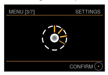
Turn the main knob clockwise to increase the brightness and anti-clockwise to decrease the brightness. Please note that the LED can not be turned off completely to facilitate showing whether the MU1 is in operation/stand-by or power off.
