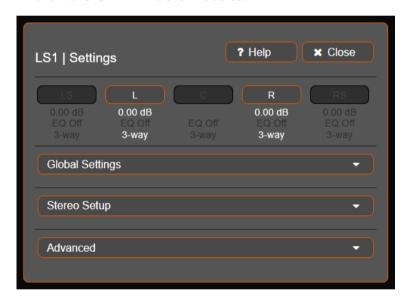
The first row shows a summary of the setup data per LS1. In the top row you see buttons with the names of the detected speakers. You can press these buttons to mute the indicated channel for a few seconds. This LS1 will blink its power LED, so you can easily identify the speaker and see if the wiring and LR switches in your system are correctly set.
