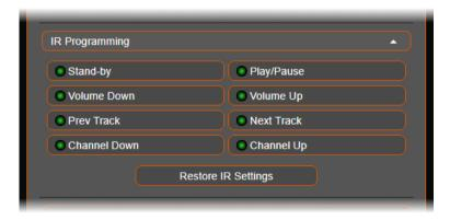
The infrared remote functionality requires an IR extension cord connected to the 3.5mm jack on the back. An extension cord is included in the packaging of the MU1.
