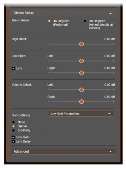
The "Toe-In Angle" should be set to follow the LS1 angles of your setup. 30 deg means 'aimed directly at listener', 45 deg means 'aimed slightly in front of the listener'. For more info about this technique, please consult the LS1 manual. This setting controls an EQ in the LS1 that corrects the high frequencies for the used angle.
