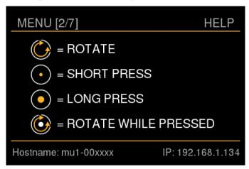
This menu shows the pictograms that are used in the MU1 for operating the main knob. At the bottom of the screen the current network information is shown. The indicated hostname depends on the serial number of your MU1. If the IP address shows "unknown", there is no network connection and in that case the MU1 cannot be found by the Streamer App in your tablet or smart phone. In that case, please check the network connection of your MU1.
