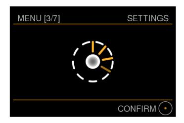
Turn the main knob clockwise to increase the brightness and counter-clockwise to decrease the brightness. Please note that the LED can not be turned off completely to facilitate showing whether the MU1 is in operation/stand-by or power off.
