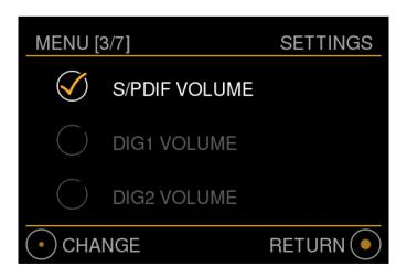
Note: volume control on the S/PDIF output cannot be enabled when there is an LS1 connected to the MU1.
