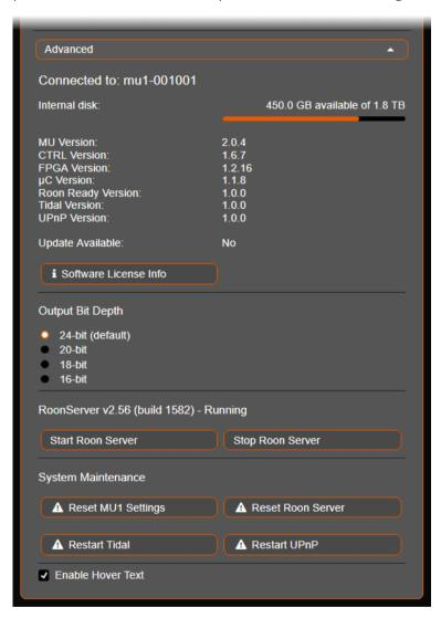
The first thing you see under advanced is the hostname of the MU1 that you are connected to, this consists of a part of the serial number.
