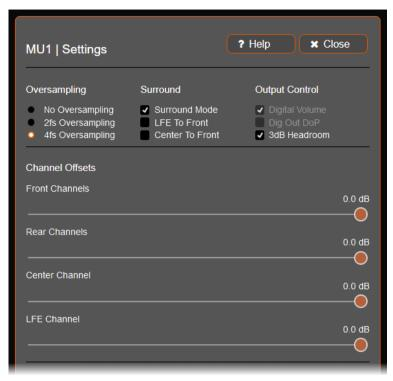
In normal mode all outputs carry the same stereo signal. In Surround Mode the LS1 and S/PDIF outputs carry the Front Left and Right channels. AES out 1 carries the Rear Left and Right channels. AES out 2 carries the Center and LFE channels. When the surround option is enabled you can give volume offsets to the Front, Rear, Center and LFE channel(s). This way you're able to match the volume difference between different speakers or DACs.
