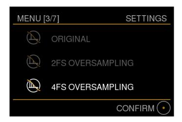
Original means that the FPGA does not touch the bits of the audio when possible. Mark that DSD rates and 8FS (DXD) will still require downsampling to 4FS, and of course the bits will be altered if digital volume control is engaged (see the next menu item).
