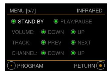
The dot will turn orange until the MU1 receives an infrared command. Press the desired button on your infrared remote to link this infrared command to the selected function. When the MU1 receives an infrared command the dot will turn green and it returns to the infrared selection menu as shown in the previous image.
