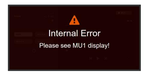
The MU1 does a self-test to guarantee the FPGA conversion quality. Whenever something is wrong it will instruct you to do a full power cycle by pressing the main dial. The unit will then shut down. Please wait until the MU1 is completely shut down, then disconnect the power cable and reconnect it. You can power up the unit again.
