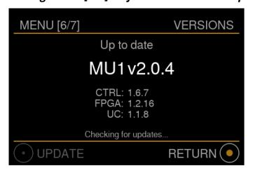
In this menu you can view the current software version and start an update. The MU1 automatically checks for an update every hour and also when entering this menu page from menu page [5/7]. If the MU1 is checking for updates, this is shown at the bottom of this menu.
