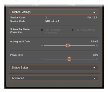
"Speaker Chain" shows how many LS1's, and in what order, are connected. The image above shows that there are two LS1's connected and the wiring goes from the MU1 to the left LS1 and then to the right LS1. In a surround setup with LS1's the indicated chain is important to double check, see the hardware manual for the proper surround setup wiring. In this chain "LS" means Left Surround and is the Rear Left channel, "RS" is the Rear Right channel, "C" is the Center channel.
