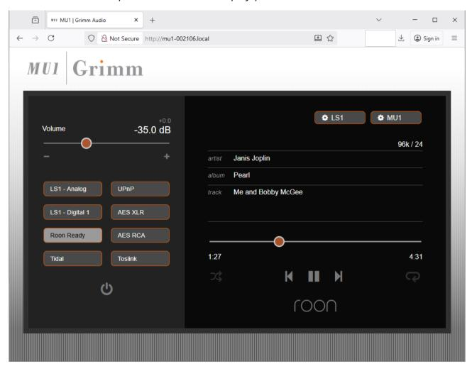
There are two sections: on the left is the control area. You can change the volume and select a source. The LS1 Analog and LS1 Digital 1 inputs are not available when you didn't connect an LS1 to the MU1. Below the inputs you can find the stand-by button.
