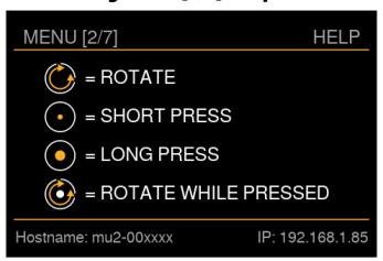
This menu shows the pictograms that are used in the MU2 for operating the main knob. At the bottom of the screen the current network information is shown. The indicated hostname depends on the serial number of your MU2. If the IP address shows 'unknown', there is no network connection and in that case the MU2 cannot be found by the Roon App in your tablet or smart phone. In that case, please check the network connection of your MU2.
