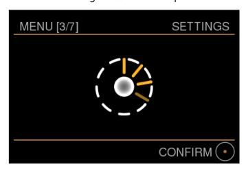
Turn the main knob clockwise to increase the brightness and counter-clockwise to decrease the brightness. Please note that the LED can not be turned off completely to facilitate showing whether the MU2 is in operation/stand-by or power off.
