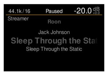
When turning the MU2 main control knob, the volume changes and the track progress bar at the bottom is temporarily replaced by a bar that indicates the current volume setting. You will hear the relays of the analog volume control clicking inside the MU2 box when you change the volume.
