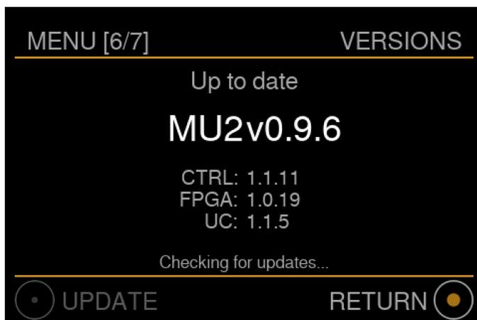
In this menu you can view the current software version and start an update. The MU2 automatically checks for an update every hour and also when entering this menu page from menu page [5/7]. If the MU2 is checking for updates, this is shown at the bottom of this menu. If your software is up to date this is indicated in the display and the bottom left icon is greyed out.
