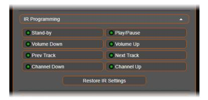
The infrared remote functionality requires an IR extension cord connected to the 3.5mm jack on the back. An extension cord is included in the packaging of the MU2.
