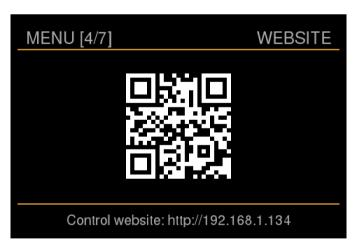
This menu shows the information you need to connect to the Grimm User Interface (GRUI). The GRUI is the web control interface of the MU2. You can scan the QR code with your tablet or mobile device. As an alternative you can manually enter the link shown at the bottom of the screen in your browser. More information about the GRUI can be found in chapter GRUI
