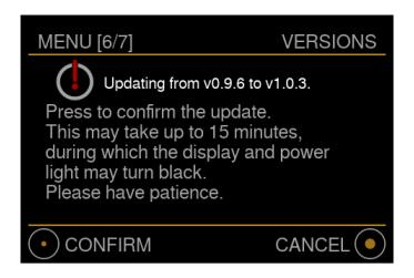
Depending on the type of update the install can take up to about 30 minutes. During this time you will not see information on the display, the power LED is fading quickly and the power button on the back is disabled.
