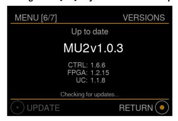
In this menu you can view the current software version and start an update. The MU2 automatically checks for an update every hour and also when entering this menu page from menu page [5/7]. If the MU2 is checking for updates, this is shown at the bottom of this menu.
