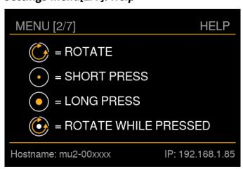
This menu shows the pictograms that are used in the MU2 for operating the main knob. At the bottom of the screen the current network information is shown. The indicated hostname depends on the serial number of your MU2. If the IP address shows "unknown", there is no network connection and in that case the MU2 cannot be found by the Streamer App in your tablet or smart phone. In that case, please check the network connection of your MU2.
