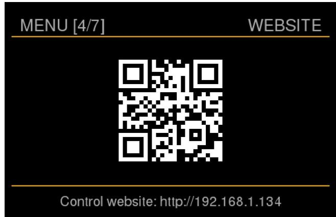
Alternatively you can enter the url link shown at the bottom of the QR page into your browser. If your router and remote device support it, you may also visit the GRUI by using the hostname instead of the IP address. The hostname can be found at the bottom of menu [2/7], it consists of a part of the serial number of your unit. Some browsers require you to add the prefix “http://” to the hostname, as in “http://mu2-00xxxxx”.
