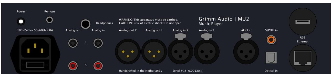
The MU2 is shipped with a proper mains power cable, use this to connect the MU2 to a mains outlet<sup>1</sup>. The MU2 works with nominal mains voltages from 100V to 240V.
