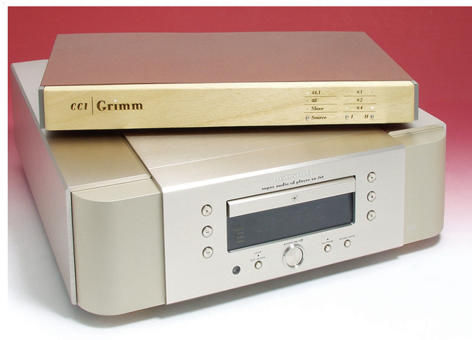
The Grimm is designed to work with CD players that have a master clock input, such as this Marantz SA-7.
