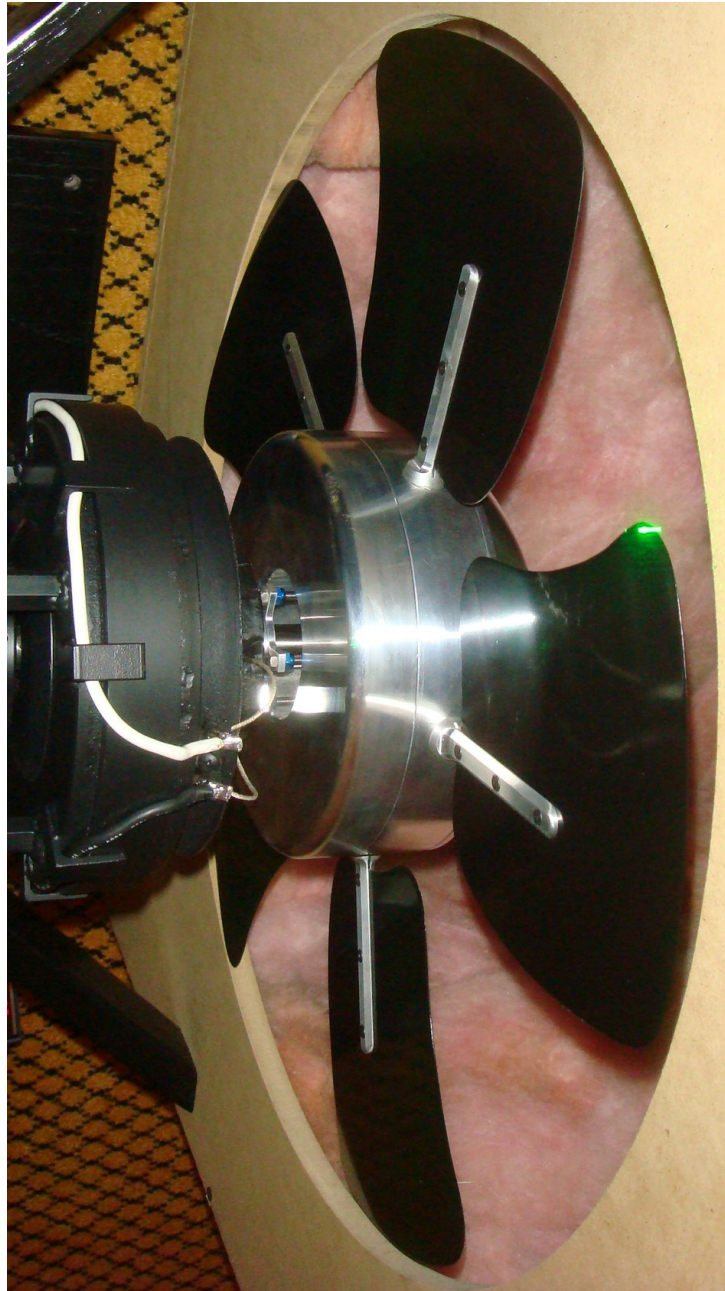
Figure 2: The Thigpen rotary subwoofer by Eminent Technology uses a fan with controllable pitch of the blades to create pressure variations between the front and the back side of the fan by changing the pitch of the blades. The back side faces a large enclosure volume, while the front side delivers the sound pressure via a second chamber covered with damping material to reduce the airflow noise.
