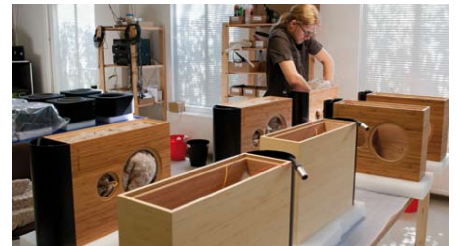
The enclosures that are purposely styled broad and flat get a sheep's wool damping, which promises best acoustical properties.
