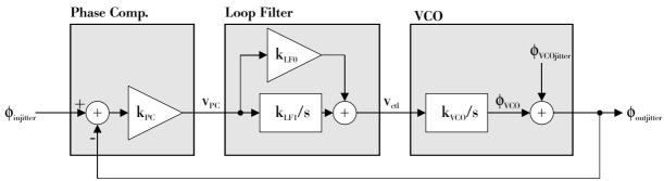
When the output  $(V_{et})$  of this integrator is constant, its input  $(V_{PC})$  is zero. When the loop is in lock, there is no phase difference between input and output.
