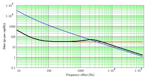
Overall, the resulting signal has less jitter than either the input signal or the VCO alone.
