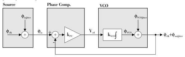
The input signal to the PLL is a clock signal of a given frequency, with a certain amount of jitter on it. We may conceive of this jitter as a varying phase shift compared to an ideal clock. Since it's only the jitter components we're interested in, we may ignore the  $\phi_{clk}$  terms and leave only the jitter terms in:
