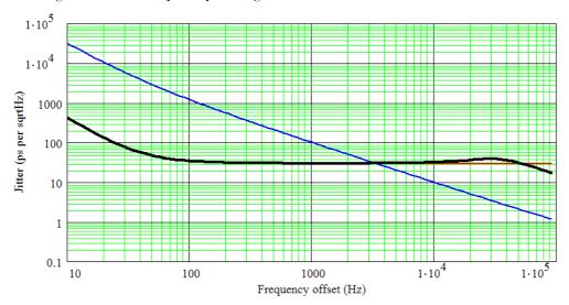
The VCO is made to follow all of the jitter of the input signal up to about 50kHz, even though left alone it would do better starting from some 3.3kHz. You see the conclusion coming: the optimal corner frequency for a given PLL and a given input signal is where the two spectra cross:
