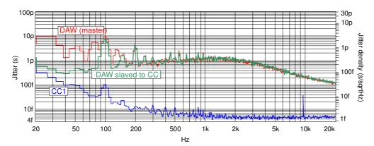
The red curve shows the jitter spectrum in master mode. Note that we already see the two-corner spectrum of a PLL system. This indicates that even in master mode, there's a PLL in the circuit. The system simply switches between an internal crystal-derived word sync reference and an external one.
