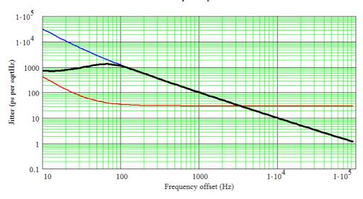
Red shows the jitter on the AES/EBU signal (I should point out that this graph oversimplifies matters a bit, representing the wideband jitter on an AES/EBU as random white noise.
