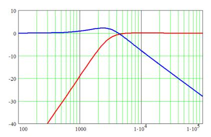
This is the transfer found in the simplest (and most common) practical PLL's. The VCO's own jitter is strongly attenuated (40dB/dec) towards low frequencies, the incoming jitter is slightly boosted around the corner frequency and is then attenuated at a rate of 20dB/dec.
