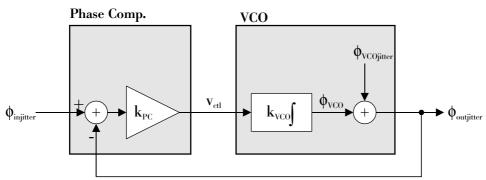
The phase comparator produces a control voltage proportional to the phase difference of its inputs and a constant factor  $k_{PC}$  (in volts per radian):
